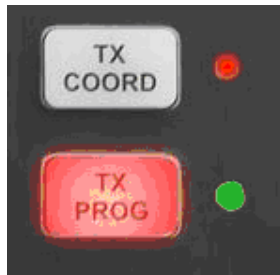
Detail of established connection in Prog Channel
