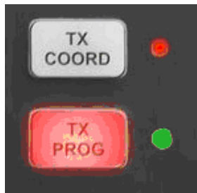
Detail of established connection in Program channel
