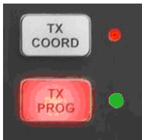
Detail of established connection in Program channel
