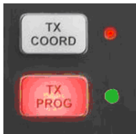
Detail of established connection in Prog Channel
