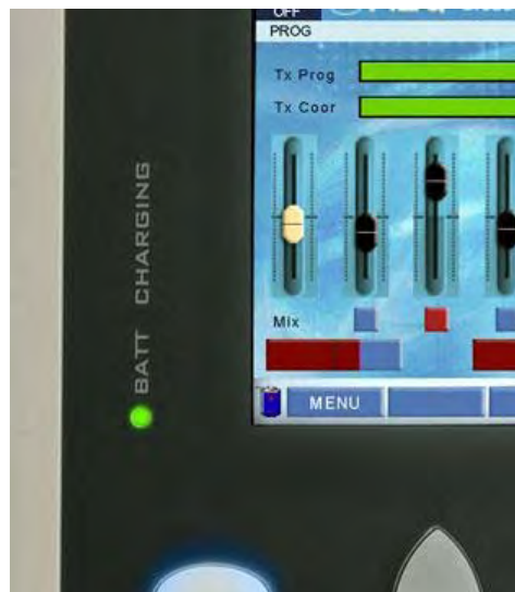
Detail of the battery charging indicator LED
