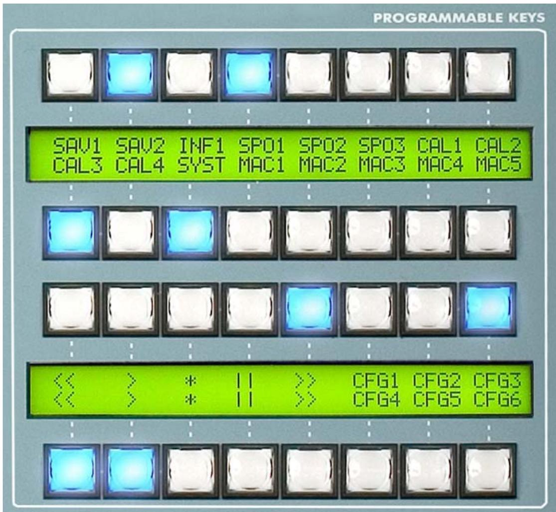
**26. Programmable Keys** have several functions that are assigned with the Console Setup software. Different functions can be set up and assigned to any of the programmable keys. Basically, the functions that can be carried out by the programmable keys are:
