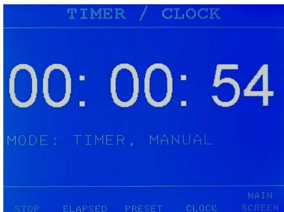
When user leaves to "MAIN SCREEN" it does not stop the CLOCK or the TIMER, in such a way that the up or down count continues.
