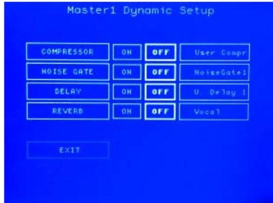
Options configured as active are indicated with the border ON highlighted and bold. Remember that **if any of the dynamic options is active (any label at ON), the “Dynamic” key for the channel will remain lit**, and will begin to flash when it is accessed this configuration display. This key will also remain lit when there is some active test signal (see section 3.2.1.4).
