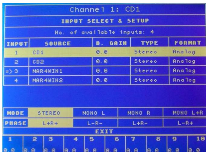
The “up” and “down” keys are used to select the source, mode or phase. When the middle button is pressed, the respective option is accessed. The “left” and “right” keys are used to select one of the available options (Mode, Phase) and the rotary encoder is used to select the source of the signal, which is indicated by means of an arrow. The option chosen is validated by once again pressing the middle button.
