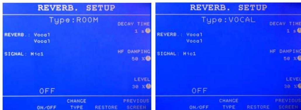
On the lower part of screen, by means of P1 through P5 pushbuttons (22) several task can be accomplished: scrolling through the different processing effects (“CHANGE TYPE”), restoring the effect to initial values (“RESTORE”) or to exit the screen (“EXIT”).
