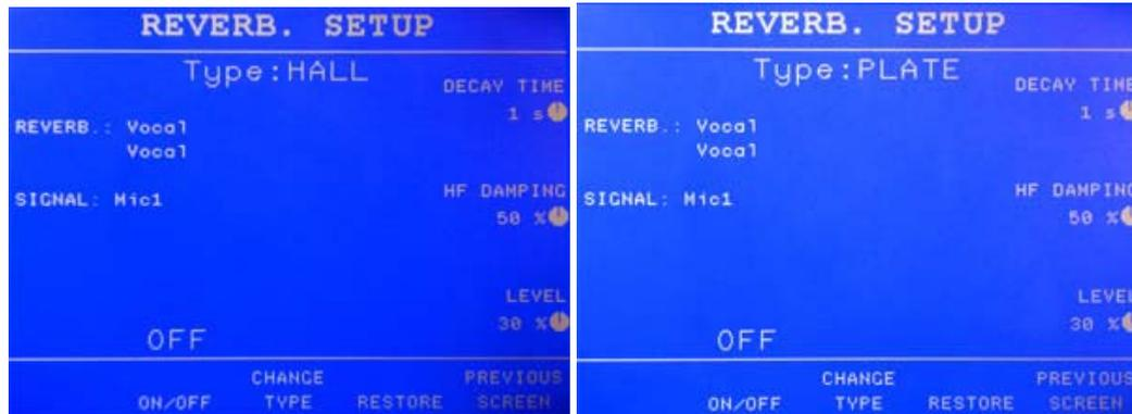
On the top of the screen all the effects available will appear (Type: Hall, Vocal, Room, or Plate). Right under “Type” and to the left are different configuration labels, which were assigned on the configuration software (the labels are used for storing a certain effect configuration). Right under that we find “Signal”, which is the audio signal to which the effect is being applied .
