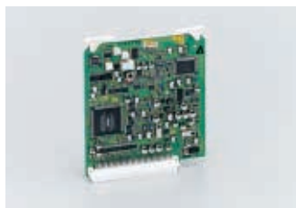
AJ-YA932G 625 Analog Video Input Board (for AJ-SD955B only)
