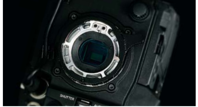
The 2/3-type bayonet mount interchangeable lens system
