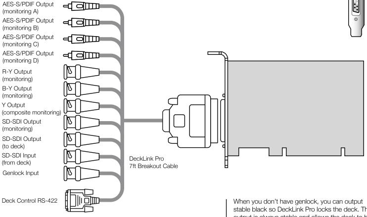
When you don't have genlock, you can output stable black so DeckLink Pro locks the deck. This output is always stable and allows the deck to be set to input reference or auto reference. Be sure to set the "Black Video Output to Deck in Capture" option to "On Digital SDI Outputs" in the DeckLink control panel, when using this feature.
