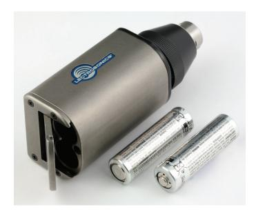
The battery compartment door is hinged to the housing and remains attached to the transmitter when opened. It securely latches in place and applies pressure to the batteries when closed. The two AA batteries are connected in series through a conductive plate on the door.
