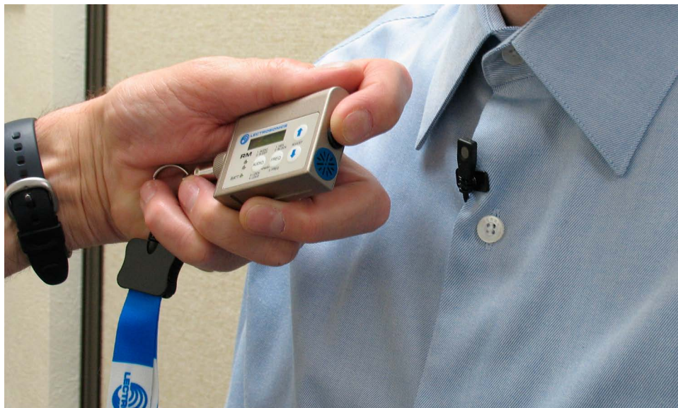
The RM should be held close enough to the microphone to change the settings on the desired SM, but not be so loud as to affect other SM units nearby.
