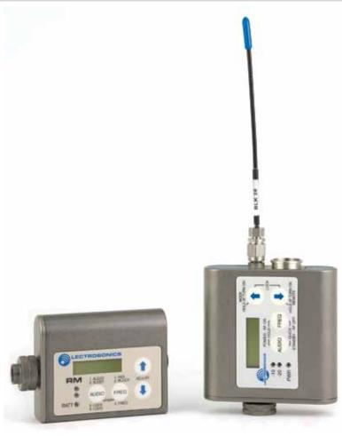
A water resistant control panel with LCD, membrane switches and multi-color LEDs make input gain adjustments, frequency and compatibility mode selection quick and accurate. The battery compartment accepts lithium or rechargeable AA batteries.
