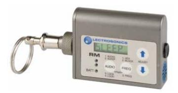
The **Lock** and **Unlock** functions on SM Series transmitters may be used to safeguard the settings and prevent accidental adjustment. When Lock mode is enabled, the switches on the transmitter control panel will not operate. The only way to unlock the controls with the transmitter itself is to remove the battery. The RM can be used to unlock or lock the transmitter controls with a brief dweedle tone while the transmitter remains in position.
