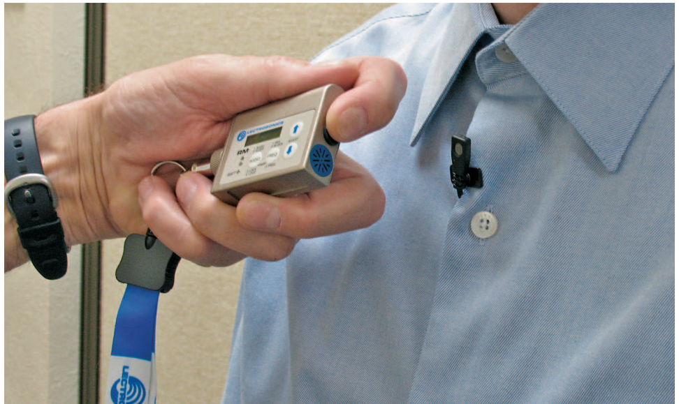
The RM should be held close enough to the microphone to change the settings on the intended transmitter, and not be loud enough to affect other transmitters nearby.
