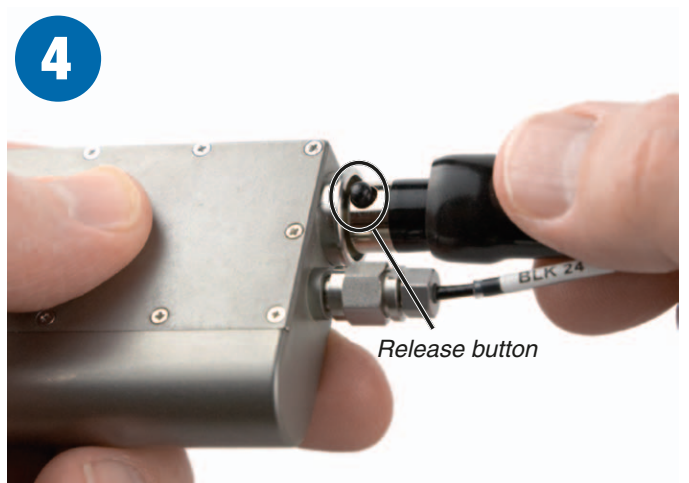
4 To remove the connector, pull the sleeve back to expose the black release button. Press the button to unlatch the plug.
