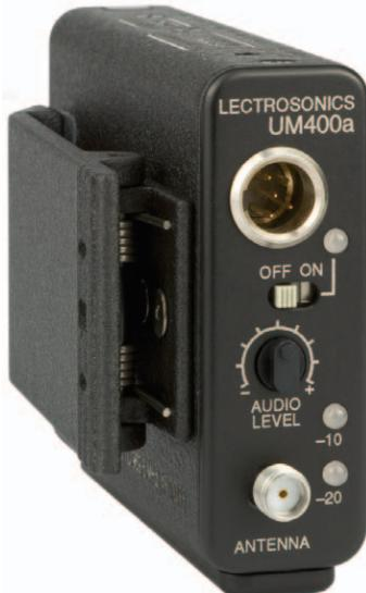
The latest digital/analog hybrid technique is presented in a classic Lectrosonics wireless belt-pack transmitter. 24-bit digital audio is combined with optimized FM to create unprecedented audio quality and RF performance. The RF transmission is an aggressively optimized FM system with +/-75kHz wide deviation for a high signal to noise ratio. The overall system delivers full bandwidth audio frequency response up to 20kHz and the operating range of the finest analog wireless systems.
